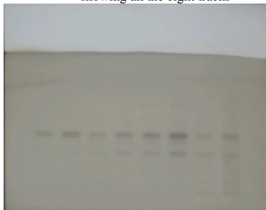
Image 1: Image of the TLC plate under white light showing all the eight tracks
